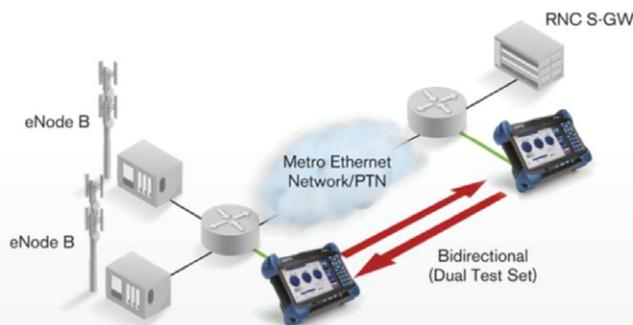
Figure 7. Dual Test Set Configuration with Bidirectional Measurements
